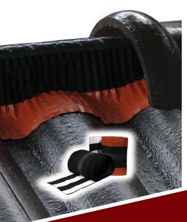
Lama Ridge & Hip Dry Fix is a solution to replace traditional wet cement mortar fixing. Its highly stretchable coated aluminium side surfaces ensures neat sealing between the ridge/ hip and the roof tiles while the water resistant fabric allows hot air trapped under the roof to exit and preventing water from seeping in. Lama Ridge & Hip Dry Fix has a self adhesive butyl backing allowing for effective self-fixing on to clean and dry tile surfaces.
